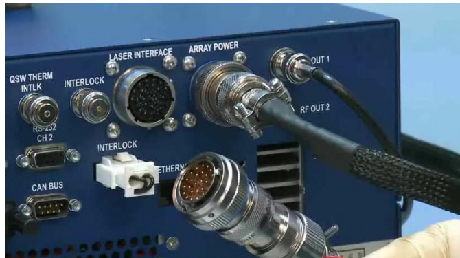
Figure 2-14. RF Signal Cable
