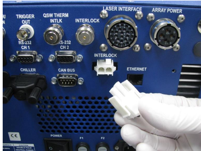
Figure 2-11. White Interlock Connectors
