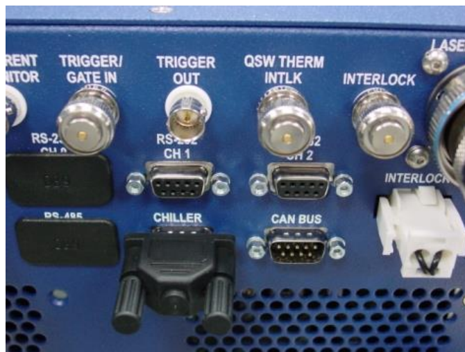
Figure 2-15. BNC Interlock Connection
