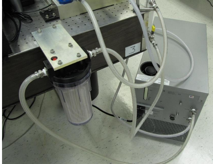
Figure 2-3. Chiller Assembled with Coolant Hoses and Filter
