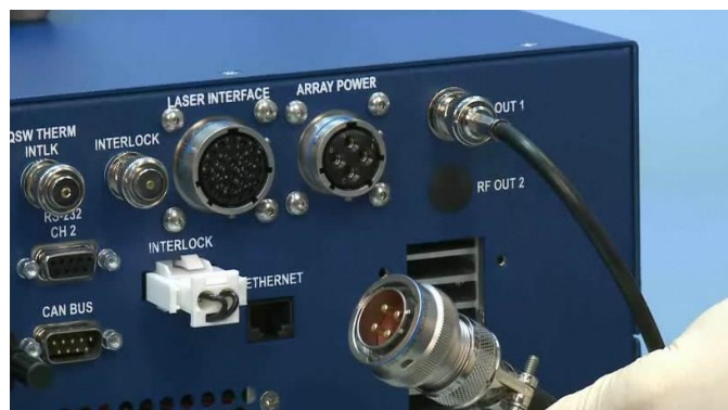
Figure 2-13. Diode Power Cable
