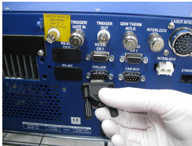
Figure 2-10. Chiller Interlock Connector
