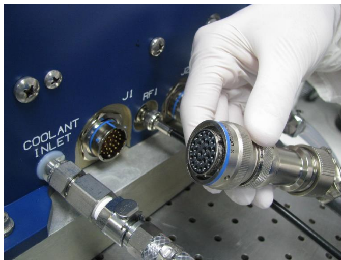
Figure 2-8. Laser Signal Connection
