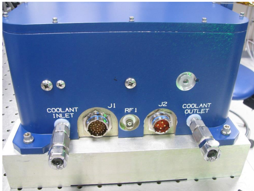
Figure 2-4. Connectors on the rear panel of the Patara EPL
